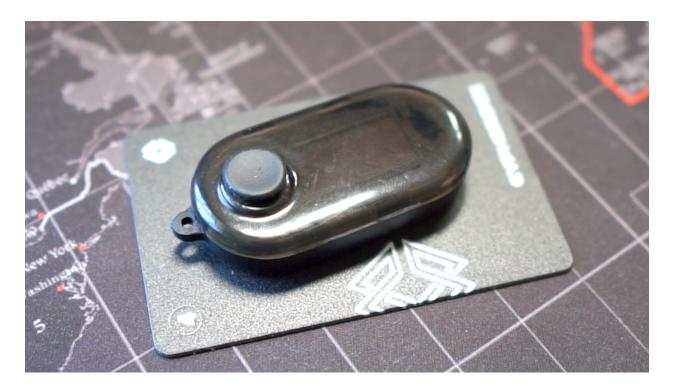
Both the case and the device PCB lack tamper evidence. For example, the device keys are not erased through opening the physical device case. The device continues to operate nominally even though the physical integrity of the surrounding case has been compromised. This helps to protect against hardware implant attacks as well as aiding in detecting evil maid attacks. Production devices will be ultrasonically welded, which will in practice make opening the device more difficult.
